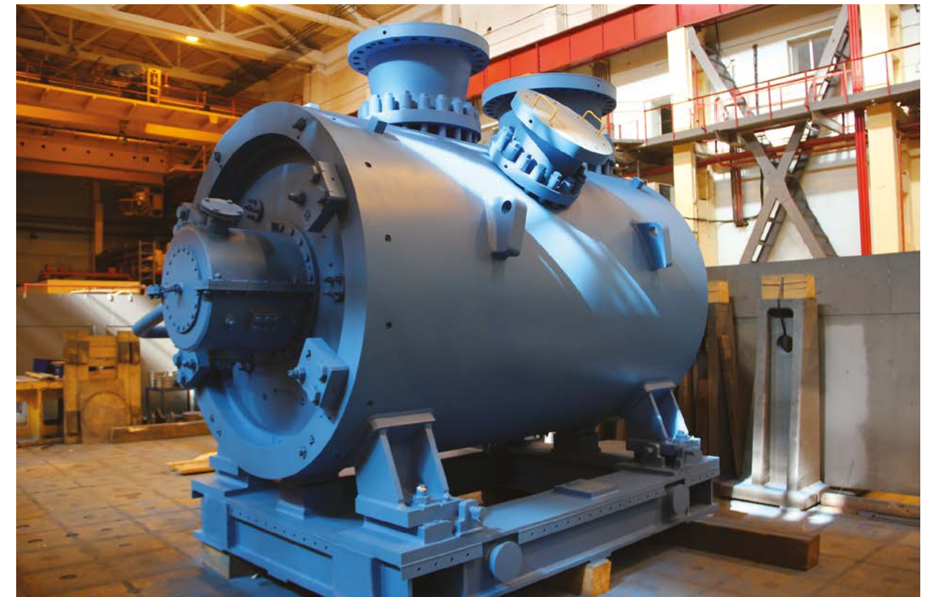
Mixed refrigerant centrifugal compressor K905-71-1C
