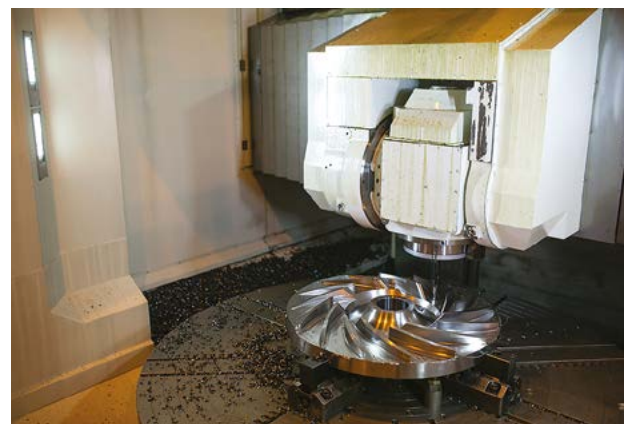
Machining of the main disc with blades of the CC impeller
