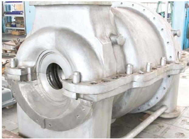
H540-41-1 compressor casing
