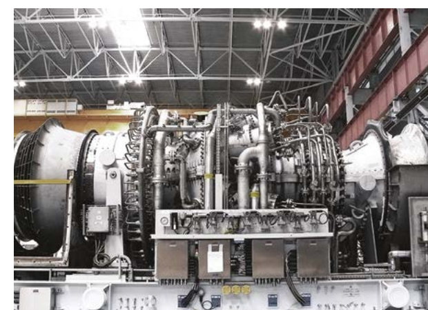
32 MW GTU on the Nevskiy Zavod production site
