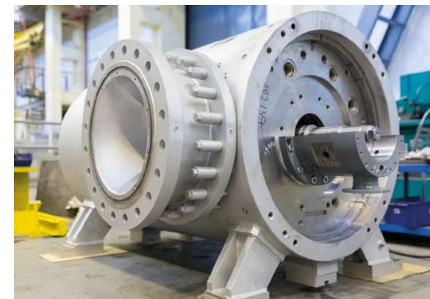
Unified casing of centrifugal compressor for T25
