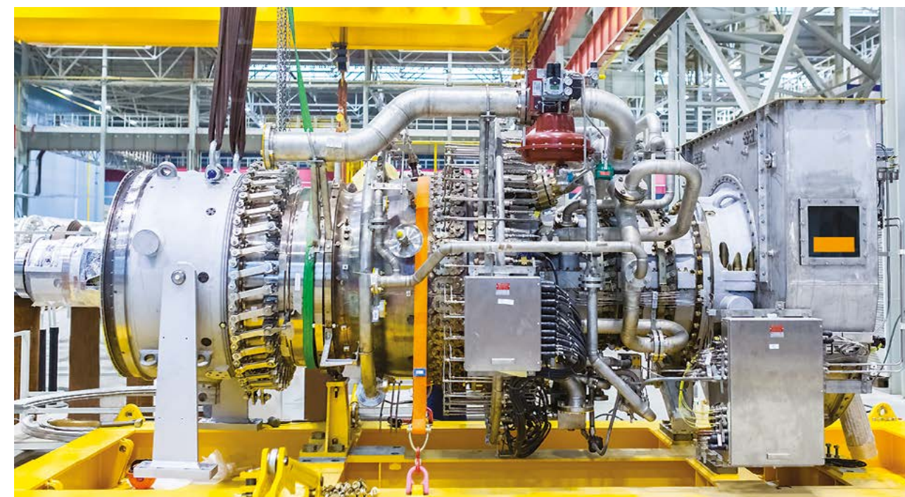
T16 gas turbine unit
