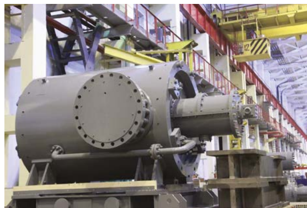
Unified centrifugal compressor 405-21-1C
