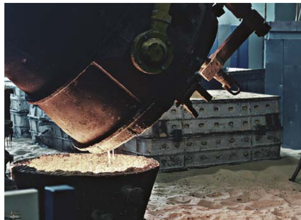
Metal casting in the melting-and-casting area of Nevskiy Zavod
