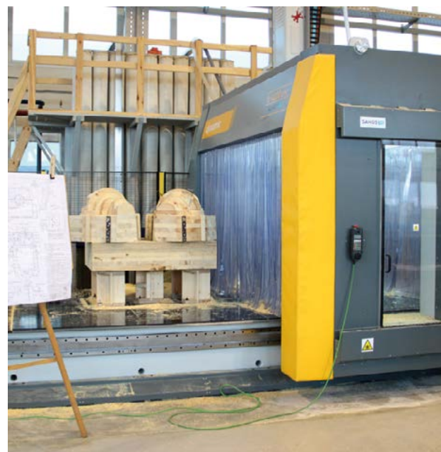
Five-axis CNC machine Dinamic FC 4000 for pattern making
