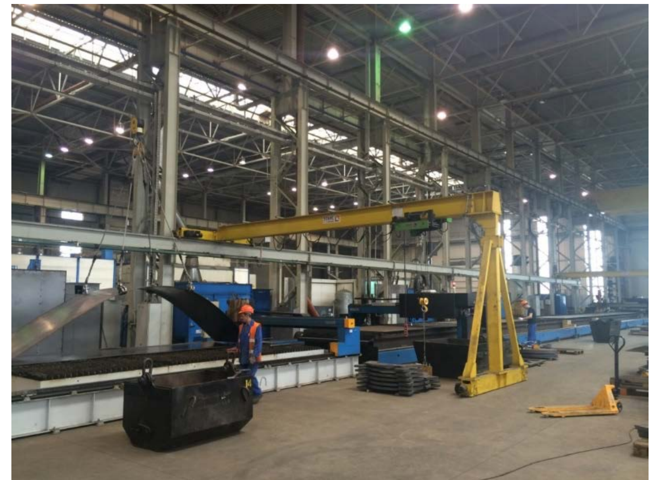
CNC gas plasma cutting machine, Nevskiy Zavod assembly-welding production area
