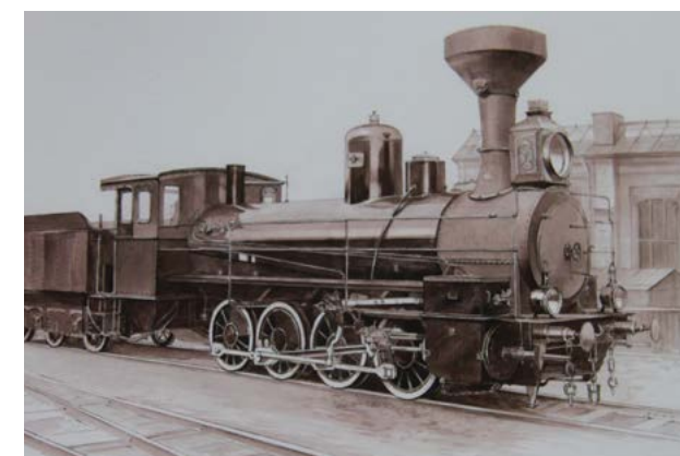
A normal-type freight locomotive with a 3-axis tender. Manufactured at Nevskiy Zavod in 1869
